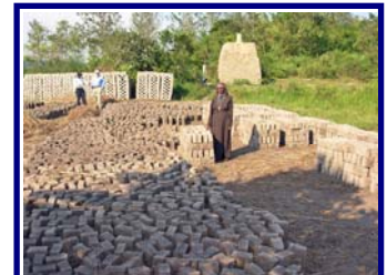
Bricks are made and fired using the clay at the school. Bricks are available to build a dormitory for the girls. Donations are needed for concrete, windows, and lighting.
