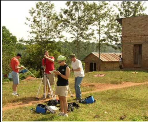
The USU team using GPS equipment to survey the terrain in preparation for designing a water supply system.
